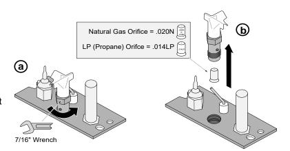
(a) Remove the manifold cover to allow access to the burner orifice (replace manifold after
