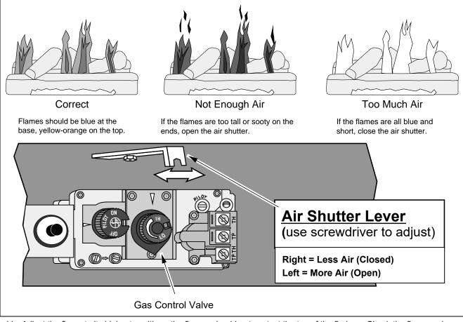
11. Adjust the flame to its highest position - the flames should not contact the top of the firebox. Check the flame on low position. The flames should burn off of each burner hole. If the heater does not work correctly, contact your Travis dealer for a remedy.
