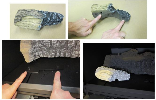
4 The right log has two holes on the bottom. Place the log so the holes fit over the two mounting studs on the right log stand.
