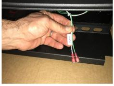
2 Connect the Green and White wires from the back of the remote to the "REMOTE" wires found in step
