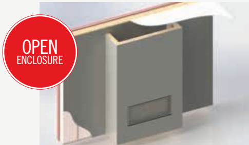
Stopping shy of the ceiling at the top, allows rising hot air to escape freely from the top of the enclosure and into the room.
